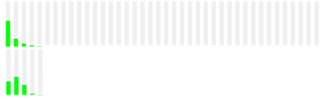
Figure 3: Hashing 2^{20} defined keys randomly distributed in a universe of 2^{24} keys into a hash table of 1.3 million keys (the load factor is 0.8). Histogram of insertion ages for open addressing (top) and Robin Hood (bottom). Gray bars correspond to very few items but are non-zero. The maximum age goes down from 46 to only 5.
